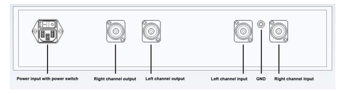
Above the mains entry you find the mains power switch. The EQU-1 can be left on permanently for maximum sonic performance. The order of left and right inputs is different from the outputs. Please note this when making connections. This is done to have equal internal wire length for both channels. The outputs can be RCA or balanced XLR on request. The GND pin can be connected to the tonearm of your turntable for lowest hum.
